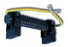
This ground coil is designed for installing in series on the equipotential bonding of two earthing systems. For example between a lightning earthing system and the masses earthing system.
