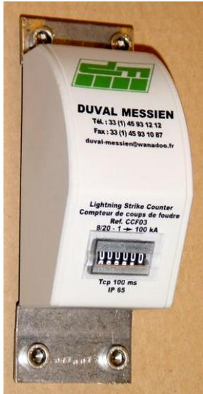
The CCF03 counter is designed to count lightning strike shocks circulating in lightning protection installation down conductors. The counter device is electromechanical and works without any power supply.
