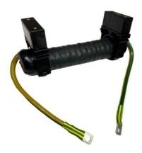
This choke is placed in series on the equipotential link of two earth connections. For example between a lightning earth connection and the earth connection of the masses.
